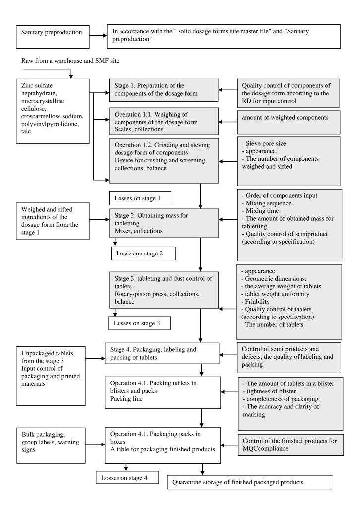
Fig.1. A block diagram of the technological process of effervescent tablets production .
