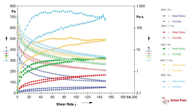
**Figure 1.** The dependence of the shear stress ( $\tau$ , Ra) of the HEC gelson the gradient of the shear rate ( $\gamma$ , s<sup>-1</sup>) and the dependence of the structural (dynamic) viscosity ( $\eta$ , Pa s) on the gradient of the shear rate ( $\tau$ , Ra).
