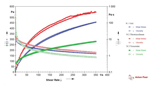
**Figure 5.** The dependence of the shear stress ( $\tau$ , Ra) of the combined gel with test composition, Troxerutin and Thiotriazolinum on the gradient of shear rate ( $\gamma$ , s<sup>-1</sup>) and the dependence of the structural (dynamic) viscosity ( $\eta$ , Ra s) on the gradient of the shear rate ( $\tau$ , Ra).
