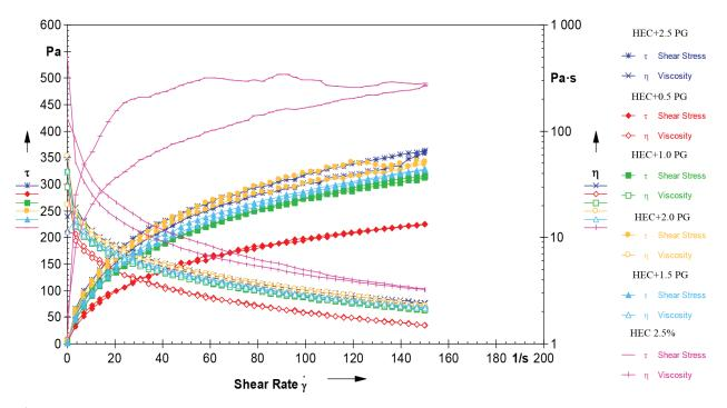
**Figure 4.** Dependence of the shear stress ( $\tau$ , Ra) of HEC gels with the PG content from the gradient of shear rate ( $\gamma$ , s<sup>-1</sup>) and the dependence of the structural (dynamic) viscosity ( $\eta$ , Pa s) on the gradient of the shear rate ( $\tau$ , Ra).
