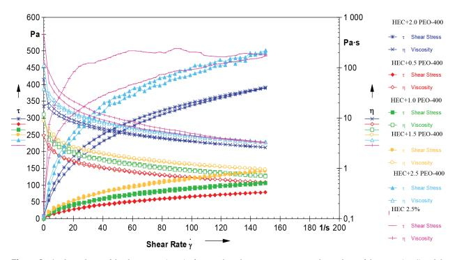
**Figure 3.** The dependence of the shear stress ( $\tau$ , Ra) of HEC gels with PEO-400 content on the gradient of shear rate ( $\gamma$ ,  $s^{-1}$ ) and the dependence of the structural (dynamic) viscosity ( $\eta$ , Ra s) on the gradient of the shear rate ( $\tau$ , Ra).
