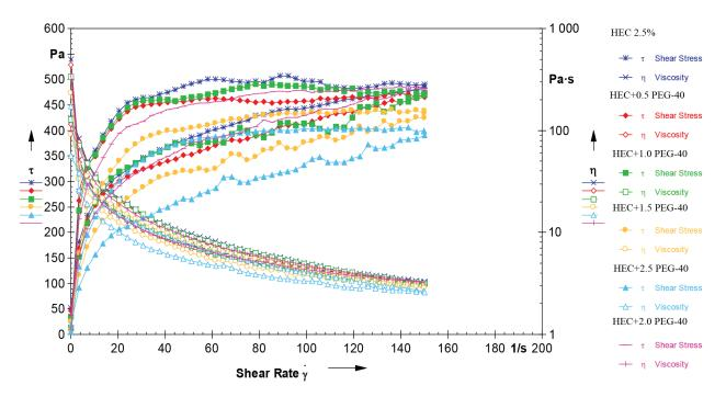
**Figure 2.** The dependence of the shear stress ( $\tau$ , Ra) of HEC gels with the content of PEG-40 hydrogenated castor oil on the gradient of shear rate ( $\gamma$ , s<sup>-1</sup>) and the dependence of the structural (dynamic) viscosity ( $\eta$ , Ra s) on the gradient of the shear rate ( $\tau$ , Ra).
