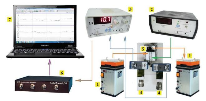
**Figure 3.** Smooth muscle preparations miographic study methodic scheme, where: 1 peristaltic pump 2 thermostat 3 amplifier 4 Capacitive tensometric sensor 5 work chamber (heated with thermostat) 6 analog-to-digital converter 7 personal computer.
