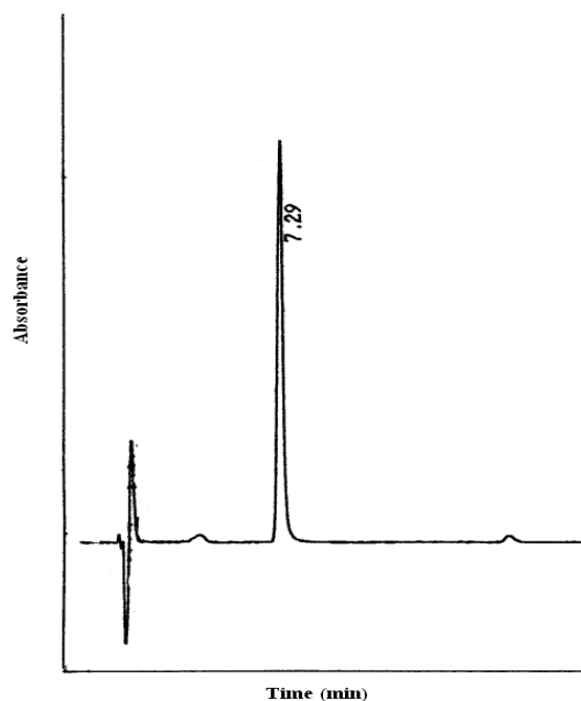
Fig. 2. Chromatogram obtained with the test solution of cream "Dermalipoin" for \alpha -lipoic acid identification
