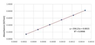
**Figure 3.** Absorbance values of chlorogenic acid as a function of the solution concentrations. The data correlation was calculated by a linear fit.
