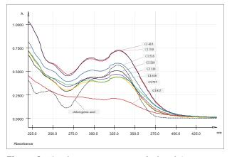
**Figure 2.** The absorption spectrum of ethanol (50 per cent V/V) chicory herb extracts for 8 sample of the raw plant material. See abbreviations in Table 3. UV/Vis absorption spectra of chlorogenic acid chemical standard at  $10.08 \mu g/ml$  in ethanol (50 per cent V/V).
