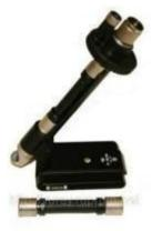
at the wavelength  $\lambda = 589.3$  nm of the sodium spectrum line D, temperature  $t = 20^{\circ}C$ , in a polarimetric tube of length l = 1 dm, and the specific optical rotation is calculated by the formula:
