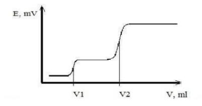
1 ml of 0.1 M perchloric acid corresponds to 23,83 мг C<sub>18</sub>H<sub>32</sub>CaN<sub>2</sub>O<sub>10</sub>. Calcium pantothenate must contain not less than 98.0% and not more than the equivalent of 101.0% bis[3-[[(2R)-2,4-dihydroxy-3,3-methylbutanoyl] calcium amino]propanoate], on a dry matter basis
