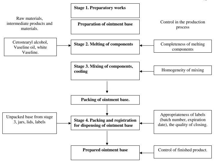
Figure 4.1 illustrates the block diagram outlining the process for preparing the ointment base.
