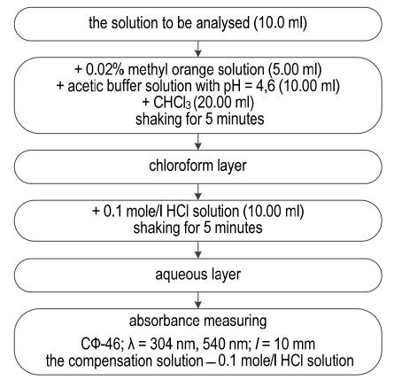
I. e. it is suggested by us to carry out decomposition of ionic associates and reextraction of methyl orange and zopiclone in 0.1 mole/l hydrochloric acid solution simultaneously and to measure the absorbance of methyl orange and zopiclone in the obtained aqueous solution by spectrophotometer.
